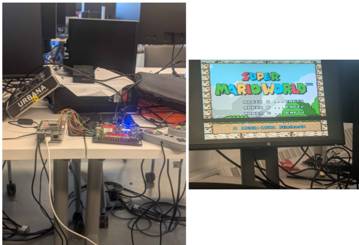
Figure 7: (left) Setup of Urbana Board connected to Pi through GPIO and USB controllers connected to Pi (right) Demonstration of Super Mario World save selection screen with this setup
